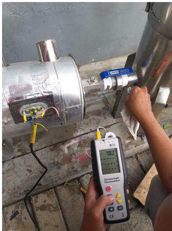
Figure 6.Purification Testing with Temperature 80°C
