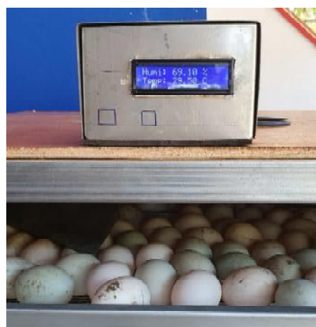
Figure 4. Control system in the hatching machine
