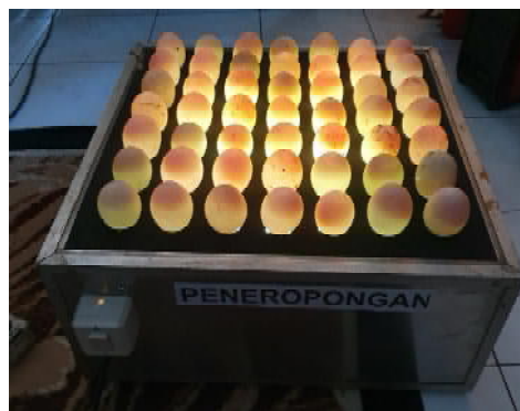
Figure 3. Candling box to select infertile eggs
