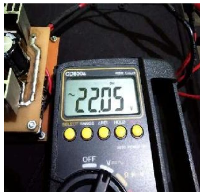
Figure 8. Motor voltage testing
