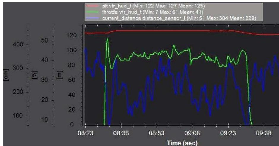
**Figure 6.** The second try UAV flight using a flight controller with barometer sensor, GPS and ultrasonic sensor
