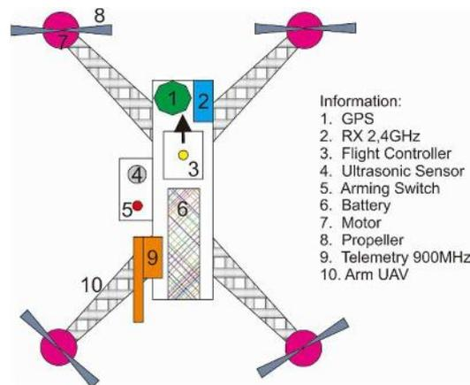
Figure 2. Full technical design of UAV with Ultrasonic sensor
