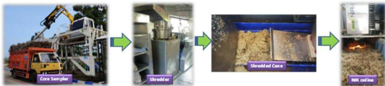
Figure 1. Core Sampler System and Shredded Cane Sample
