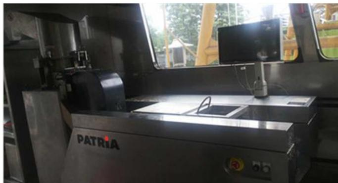
Figure 2. Automated Cane Analyzer with NIR Instrument for the evaluation of sugarcane quality
