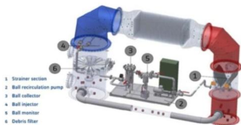
Gambar 3. Ball Cleaning Condenser (Qodir, 2014)
