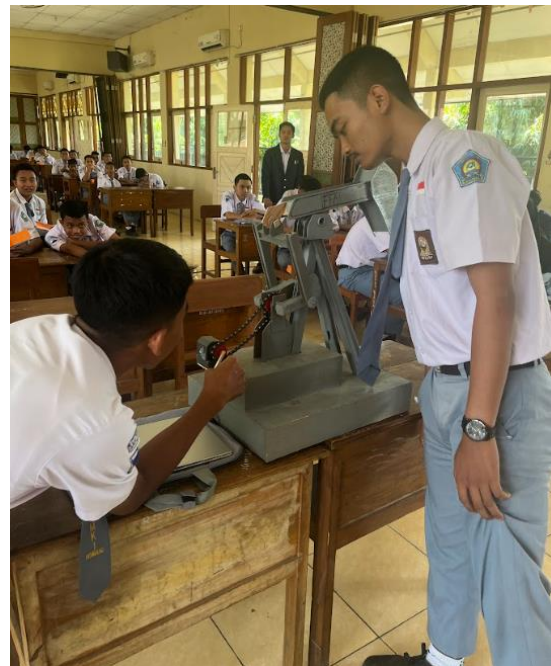
Gambar 4. Demonstrasi Peraga Alat sucker rod pump
