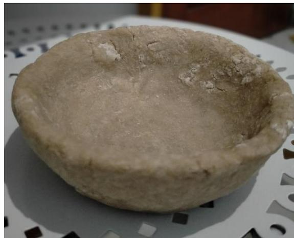
**Gambar 8.** *Prototype mangkok biodegradable foam*
