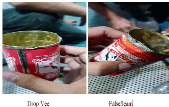
Gambar 3. Defect drop vee dan false seam
