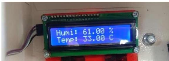
Gambar 6. LCD 16x2
