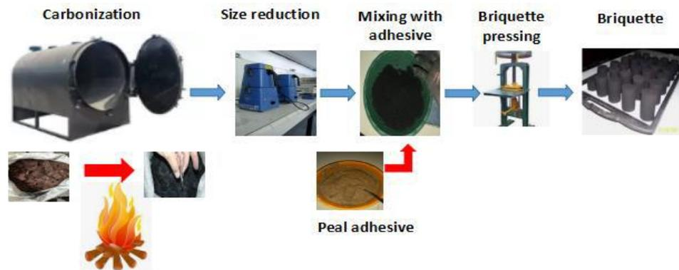
Figure 3. Bio briquette preparation schematic diagram
