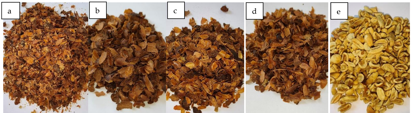
Figure 4. Raw HS (a) ; Sorted HS of size 7.5mm (b), 6.5mm (c), 5.5mm (d), and pixel (e).
