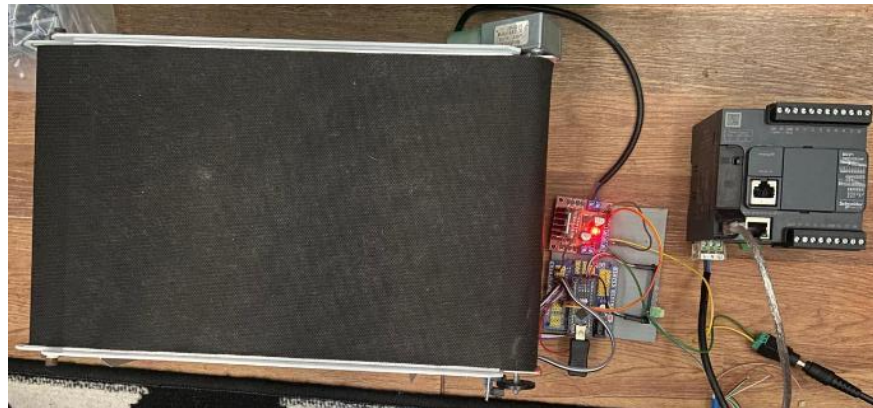
Figure 3. Conveyor and controller devices
