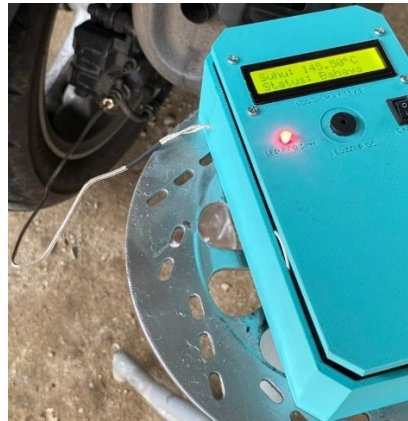
Figure 4. Application of Temperature Measurement And Monitoring Systems In A Motorcycle
